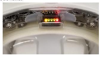
**Be certain that the Battery** being used to test the suspect Helmet does indeed power up another Helmet and that on another Helmet all 5 LEDs are lighted by that Battery.
