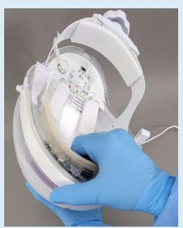
Before proceeding, ensure the Power Cord is aligned with the Liner Power Cord Slot.
