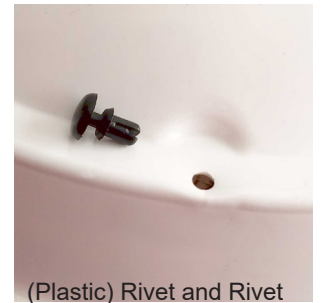
(Plastic) Rivet and Rivet Hole to be filled.
