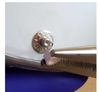
3. Continue to tilt/twist the pliers and pull forward until the Rear Adapter is off the Helmet.
