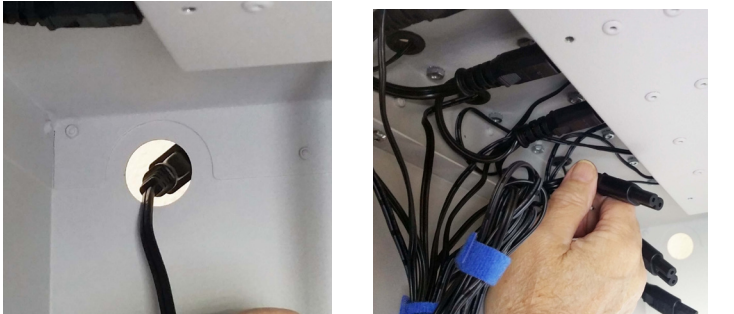
6. From inside the Cart, pull the Power Cord through the Cart Cord Opening.
