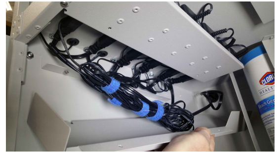
6. Ensure the new Power Cord is fully out the back of the Cart, compact the Cord Bundles, and replace the Gang Charger Cover Bracket.
