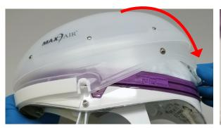
2. Hold the Helmet/Liner/ Filter Cartridge upright by its rear underside with one hand, insert the Helmet Front Adapter into the inside of the FCC Front Adapter, and pull the FCC, back, over and down onto the Helmet.
