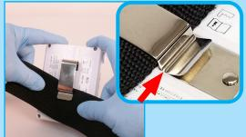
1. Place a fully charged Battery's over the Belt with the Clip Detent touching the Clip, Metal-to Metal.
