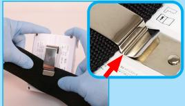
1. Remove a fully charged Battery from the Charger and place the Belt 2. Place the Belt comfortably around the waist fully under the Battery Clip so that the Clip Detent touches the Clip, Metal-to Metal.
