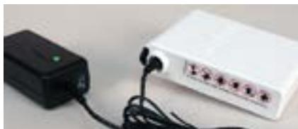
1. Obtain a fully charged battery. (Charger LED should be green after battery is connected to charger for more than 10 seconds.)
