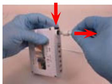
Disconnect the Helmet Power Cord from the Battery - push the Secure Connection Button down, pull Cord Connector out, release the Button.
