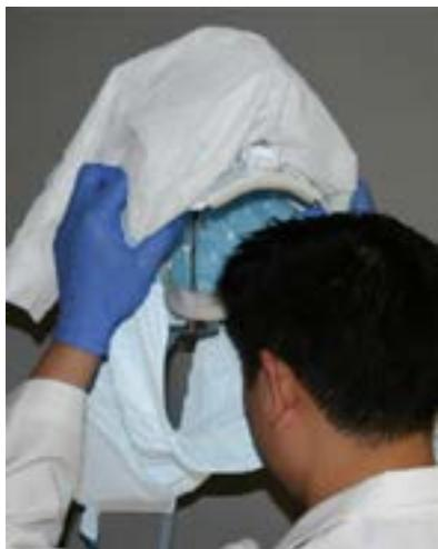
1. Flip the back side of the Filter Hood up and over the Helmet to the front. Grasp the Helmet on each side with the Filter Hood Lens facing the floor and the Rotary Adjustment Knob facing the ceiling.
