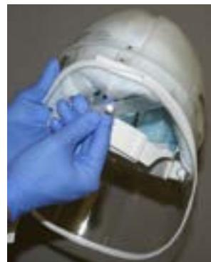
5. Secure the Filter Cover to the Helmet in the back by pulling the straps under the back of the Helmet and snapping them together.
