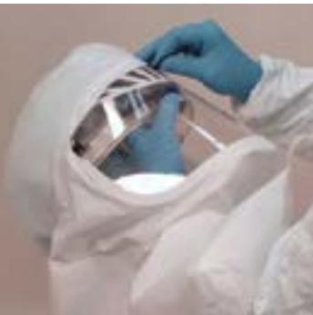
3. Pull the Filter Hood over the front end of the Helmet.
