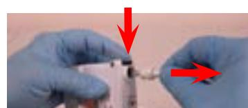
Disconnect the Helmet Power Cord from the Battery - push the Secure Connection Button down, pull Cord Connector out, release the Button.
