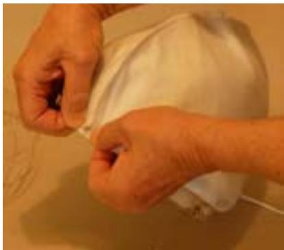
3. Pull the Filter forward and place the Filter Front Alignment Hole over the Helmet Front Alignment Post .
