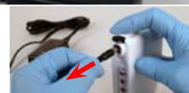
1. Connect the Charger (single and/or 6-Gang) to an appropriate grounded wall mains power source (120-240 VAC, 50-60 Hz) before connecting to the Battery(ies). The Charger green status LED should turn on.
