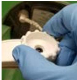
4. Turn the Headband Ratchet Knob counterclockwise to loosen Headband for ease of donning Helmet.
