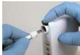
11. Disconnect the Helmet Power Cord from the Battery - Press down on the Secure Lock (Black) Button to release, then pull the cord connector out from the Battery connection receptacle.
