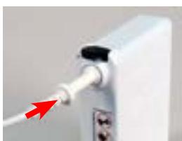
To initiate air-flow, connect the Helmet Power Cord to the Battery. Push the Power Cord Connector into the Battery Receptacle until the Secure Connection audibly clicks.
