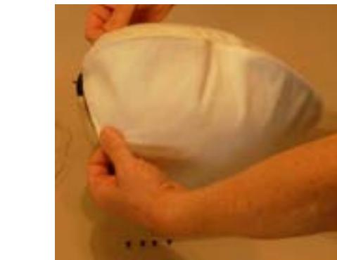
1. Tuck the rear of the Filter up under the Helmet back; pull the Filter forward over the Helmet.
