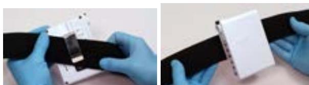
2. Assemble the battery onto the belt. Place the top edge of the Belt under the Battery Clip. Move the Belt fully under and up to the top of the Clip.
