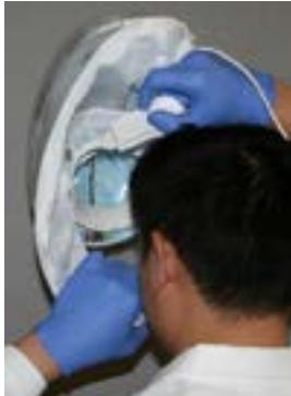
1. Adjust the Helmet Rotary Adjustment Knob counterclockwise to insure the headband will easily fit over the head.
