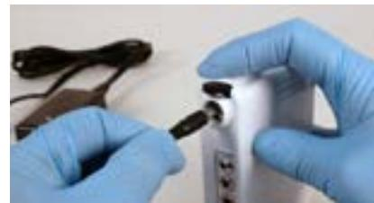
12. Connect a powered on Battery Charger connector to the Battery. Push connector into Battery receptacle fully - Do NOT push down on the Battery Secure Lock (Black) button.
