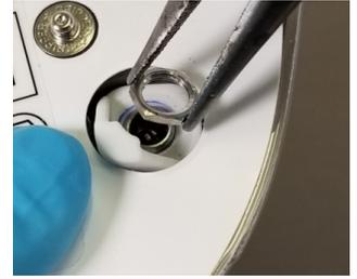
4. Turn Hex Nut until it is loosened away from the Power Jack and remove completely from the connection.
