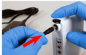
10. With Charger connected to safe power source, connect Charger Cord to the Battery. Push Charger Cord Connector into Battery Receptacle until fully seated.
