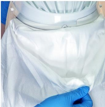
4. Grasp the back of the Hood Filter and begin to pull the Hood up and over the Helmet.
