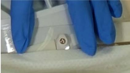
1. Attach (snap) center Hood-Lens mounting hole over Helmet center mounting post.
