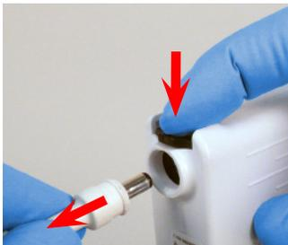
9. Disconnect the Helmet Power Cord from the Battery - Press down on the Secure Lock (Black) Button to release, then pull the cord connector out from the Battery connection receptacle.
