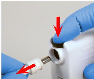
00. Disconnect the Helmet Power Cord from the Battery - Press down on the Secure Lock (Black) Button to release, then pull the cord connector out from the Battery connection receptacle.
