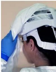
5. Unsnap each side attachment and continue moving rolled Hood forward and off front Helmet Mounting Post.
