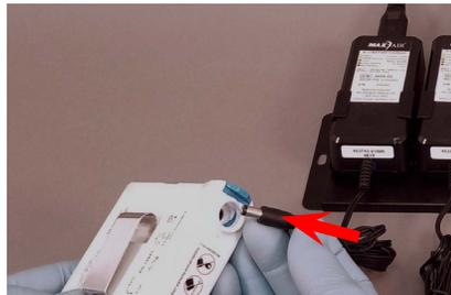
2. Connect the Battery(ies) to the Charger(s) by pushing the Charger Cord Connector into the Battery Connector Receptacle until fully seated. The Charger LED should change from Green to Yellow or flashing Yellow to indicate charging. If the LED is Green after being connected to the Battery for 10 seconds, the Battery is ready for use.
