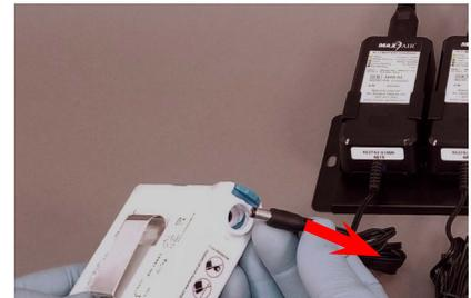
3. The Charger LED changes to Green when charging is complete. Disconnect Battery(ies) from Charger(s): pull the Charger Cord Connector from the Battery Connector receptacle. The Battery(ies) is(are) ready for use.
