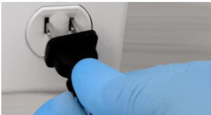
1. Connect the Charger to an appropriate grounded wall power source (120-240 VAC, 50-60 Hz) before connecting Battery(ies). The Charger Green status LED should be blinking.
