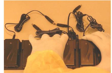
D. Hold the bracket securely in one hand with the charger clips towards the top. Begin sliding a 2600-01 Charger into an empty charger clip, with battery connection cord towards the top.
