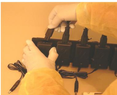
G. Connect one of the six extensions of the Charger Power Cord securely to the Power Cord Connector on one Charger.
