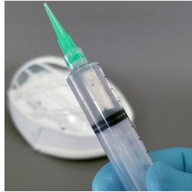
1. Place some Clear Gorilla Glue in the Syringe; 0.5 cc to 1.0 cc should be sufficient.
