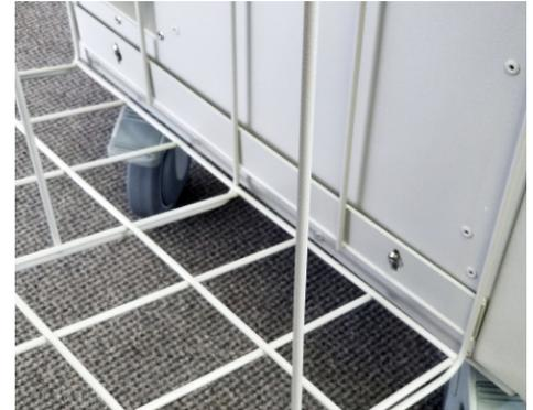
3. Slide the Rack Mounting Slots over the Mounting Screw heads and then down onto the Screw threads.
