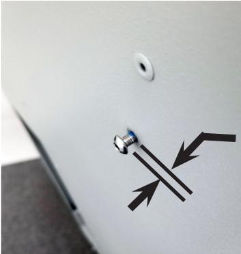
1. Un-screw each of the four Rack Mounting Screws on the side of the Cart so there is approximately 1/4 inch of thread showing.
