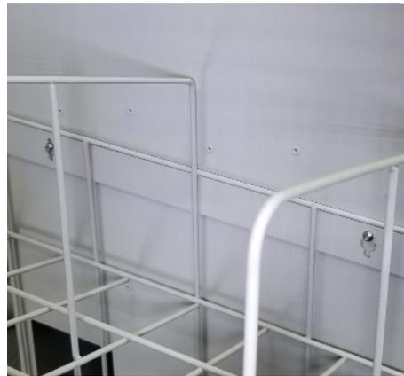
2. Slide the Rack Mounting Slots over the Mounting Screw heads and then down onto the Screw threads.
