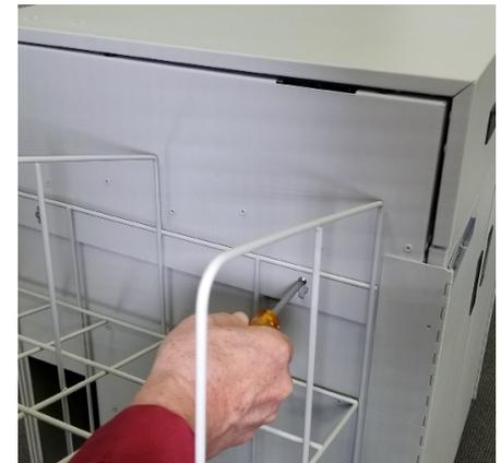
3. Tighten all four Cart side Mounting Screws to secure the Rack to the Cart. Tighten securely without over tightening.
