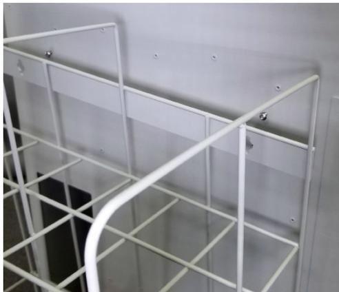
4. Move the top of the Rack to align its top Mounting Slots with the top Cart Mounting Screws.
