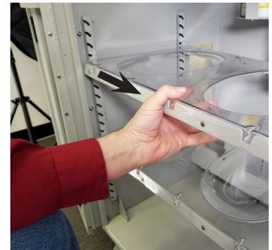
3. Continue to move the Shelf backward and then downward until the Shelf Pins are fully secured in the furthest back and down Slot positions.
