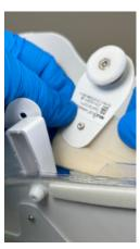
2. Place one Hanger attachment hole over the snap on the Front Strap and snap them together securely.
