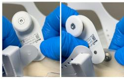
1. For one side Hanger, unsnap the Side Strap off that Hanger and remove the Hanger off the Front Strap.
