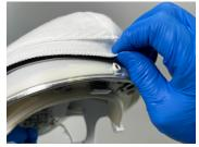
2. Lift up the front of the Filter and unsnap it from the Cage front Snap Hole.
