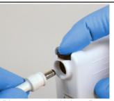
2. Disconnect the Helmet Power Cord from the Battery - Press down on the Secure Lock (Black) Button to release, then pull the cord connector out from the Battery connection receptacle.
