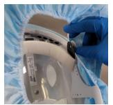
2. Lift each side of the Gaiter up and off each side Hanger.
