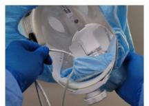
1. Pull the entire Power Cord back though the Gaiter back Button Hole.
