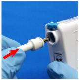
1. Connect the Power Cord connector to the Battery. 2. Push Power Cord connector in to the Battery Con-Do NOT push down on the Battery Secure Lock (Black) button.
