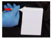
2. Connect Helmet Power Cord to Battery; push Power Cord Connector into the Battery Receptacle until the Secure Connection audibly clicks.
