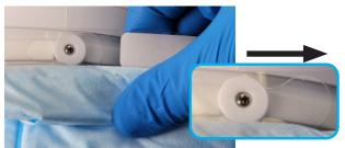
1. With the blank side of the Bonnet Label facing forward of the Helmet, place the circular end of the Bonnet Lens front Mounting Hole over the Helmet front Mounting Adapter, then slide the lens all the way to the (wearer's) left side.
