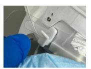
5. Detach right (wearer's) Lens side from Helmet by lifting the Lens Hole bottom down, out, and up off that side Helmet Mounting Adapter, and remove the Bonnet completely from the Helmet. Discard the Bonnet as contaminated waste.
